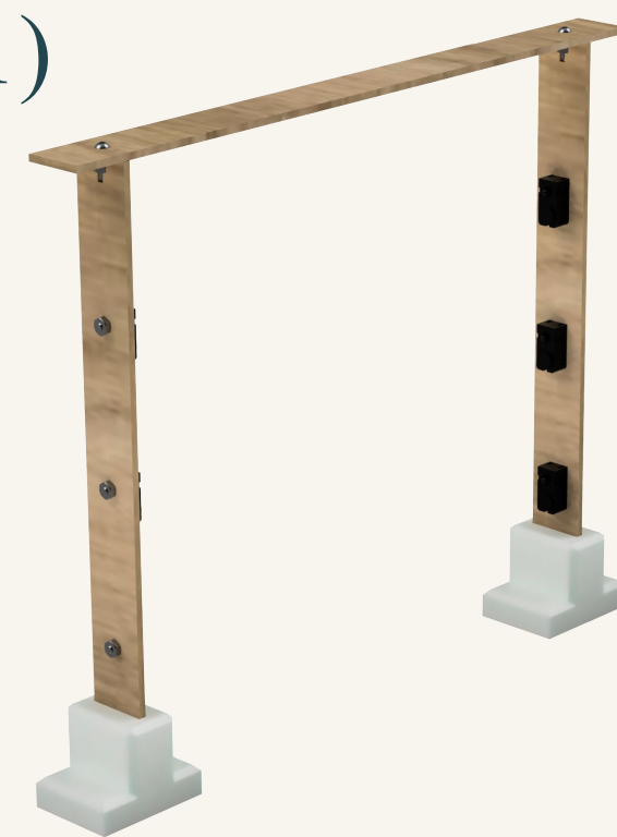
Figure 1 (above): Prototype (10 × 10 in.) was designed in Autodesk Fusion and constructed using 3 mm plywood and 3D-printed holders.
