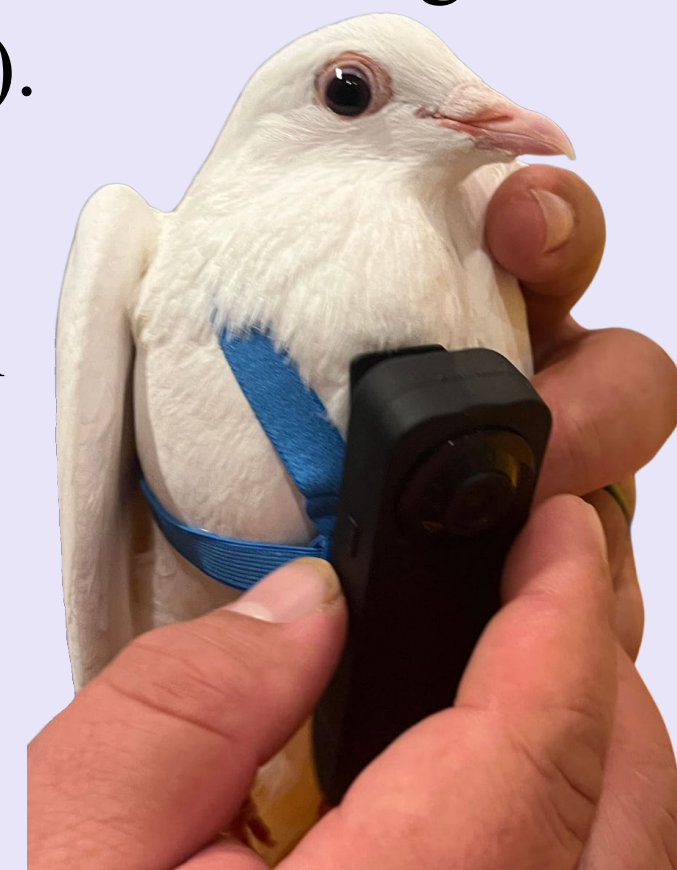
Figure 2 (right): In initial fittings, the camera was too big, resulting in restricted movement.
