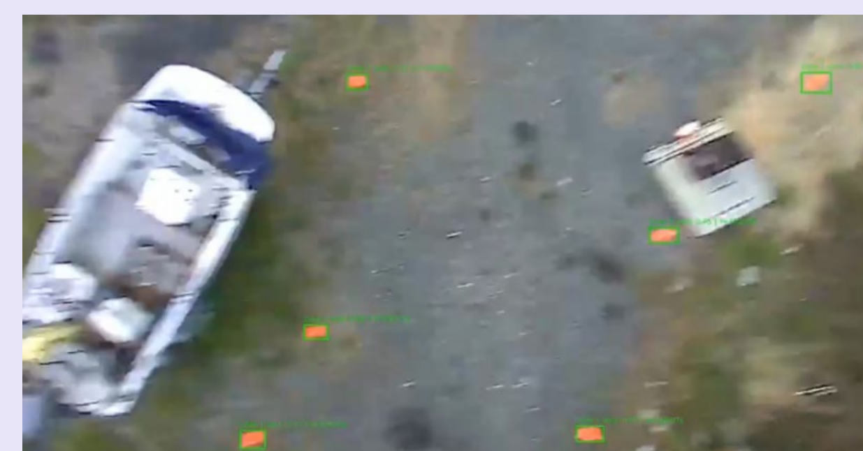
Figure 5 (right): Video footage was taken off the camera's SD card and uploaded into the software, once processed, cones detected on video were highlighted by a green box around them.
