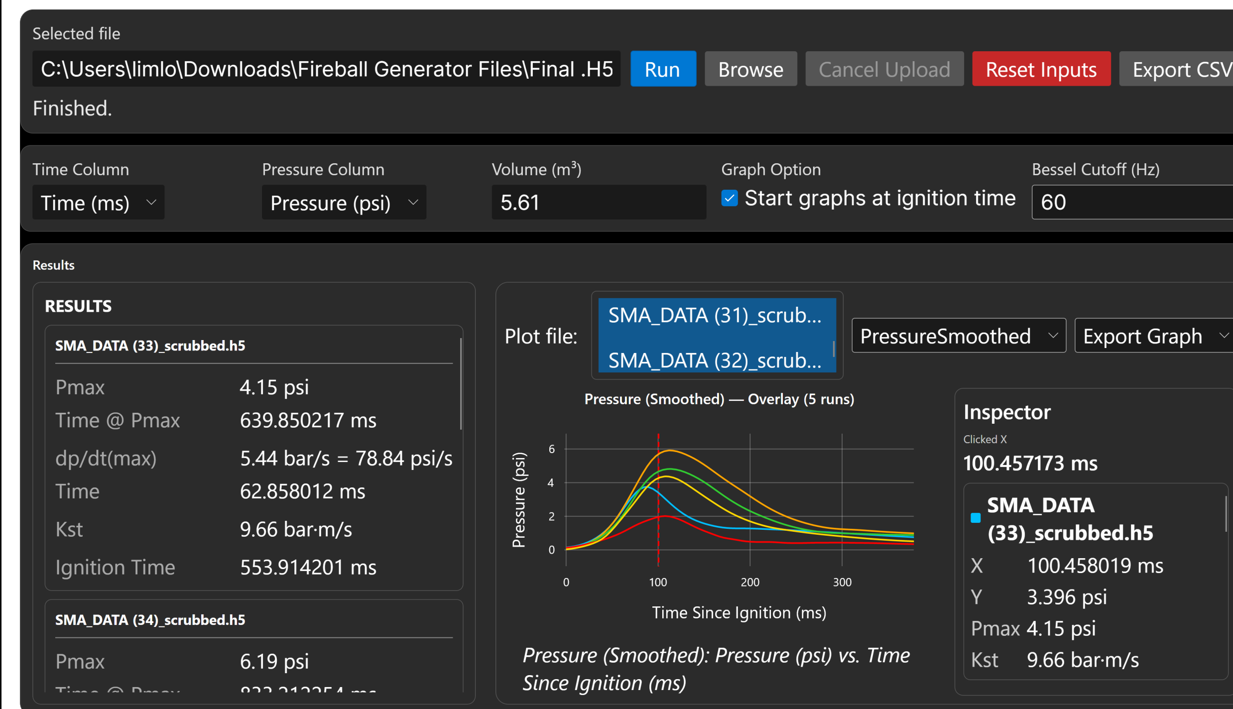
Figure 2 (above): The K_{st} Analyzer reads .h5 files generated by ATC sensors and has raw, smoothed, derivative, and integral graphing, as well as multiplot capabilities.
