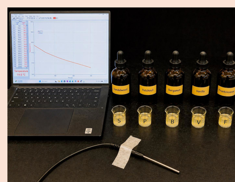
Figure 1: The experimental set up consisted of five 10 mL beakers containing perfume and sweat mixtures. A temperature probe was wrapped in circular (15 cm diameter) filter paper and held in each mixture for ten seconds. During each trial, the probe was secured by a piece of tape to minimize experimental error. A laptop was used for running Logger Pro that measured the rate of evaporative cooling. The documented rate used for data required a linear fit feature in Logger Pro to analyze the same 20–40 second interval for each trial.
