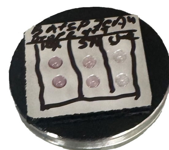
Figure 1 (left): Aluminum-coated microscope slide mounted on a circular SEM holder. Each column is a concentration (10×, 5×, and 1×) and each row is an exposure time. The holder ring has a diameter of one inch.
