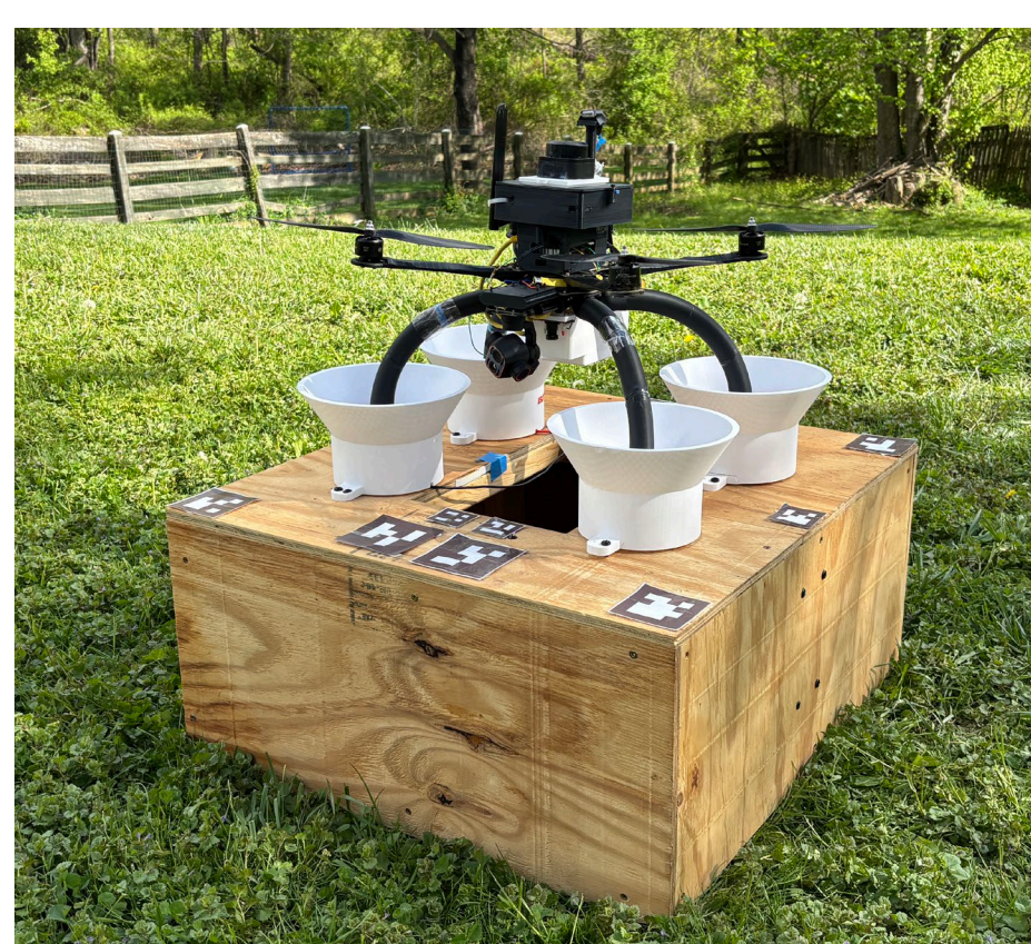
Figure 3 (right): Aircraft landed atop its compatible charging base station.
