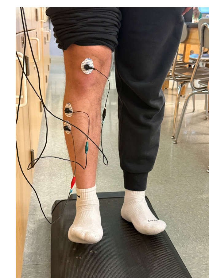
Figure 2 (left): Electrode and lead wire placement used to record EMG activity from the gastrocnemius medialis during the calf raise exercise.
