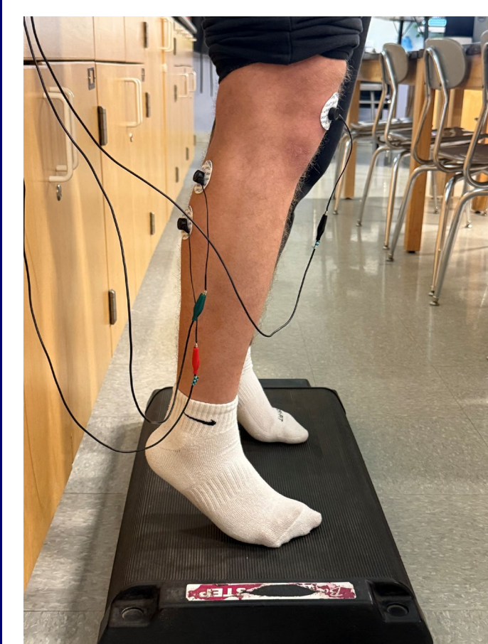
Figure 2 (left): Electrode and lead wire placement used to record EMG activity from the gastrocnemius medialis during the calf raise exercise.
