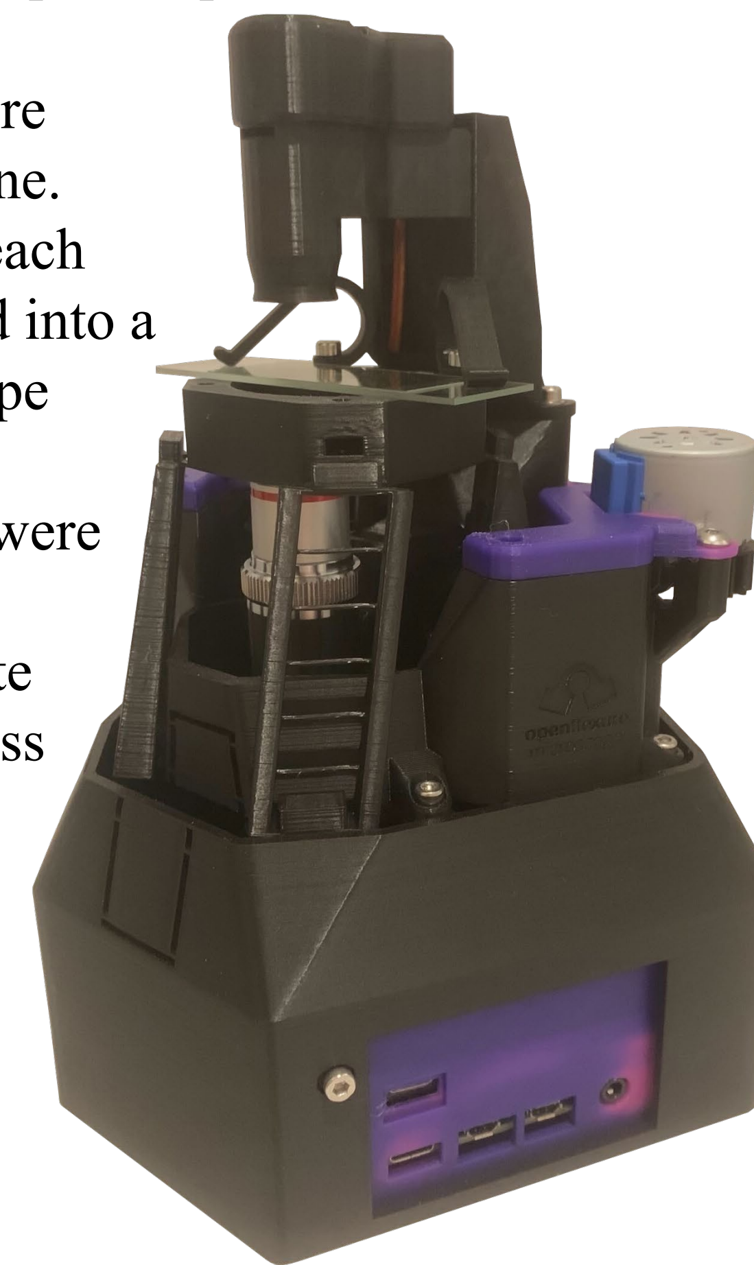
Figure 2 (right): The OpenFlexure Microscope is controlled by the stepper motors in the back, and has the objective lens and camera underneath the sample. The electronics drawer is printed in thermochromic filament to warn of potentially dangerous heat. Dimensions are approximately 145 × 132 × 256 mm.
