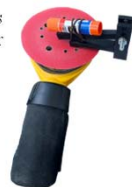
Figure 2 (left): A constant force was applied onto samples for 60 seconds at speed 6 on a DeWalt sander.
